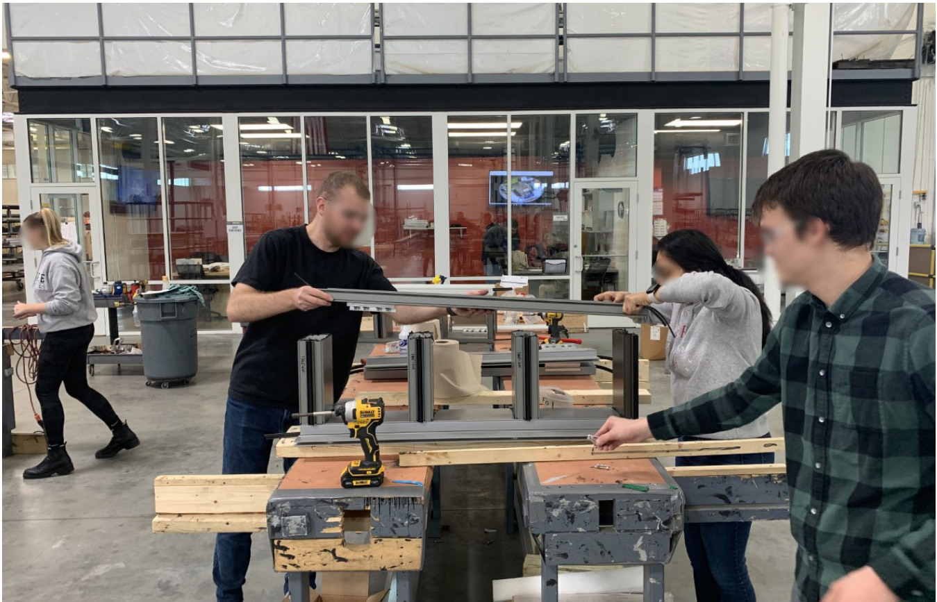
Figure 10. Students assembling a unitized curtain wall unit in manufactures shop. Image by author.
